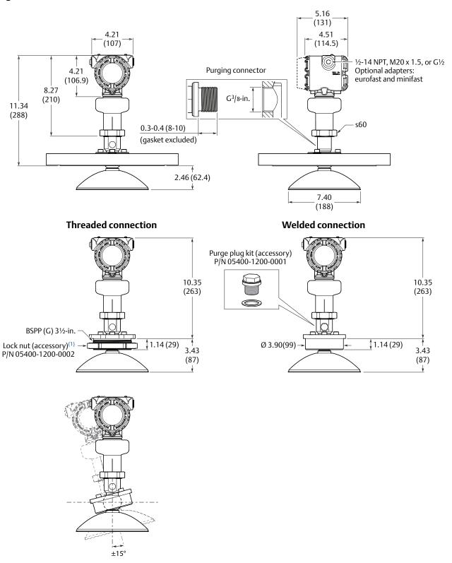
1. Maximum flange thickness (with lock nut): 0.59 in. (15 mm) Dimensions are in inches (millimeters).
